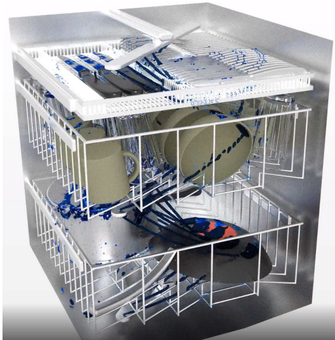
Figure 5. Fluid management in dishwasher (VOF-film-LMP).
